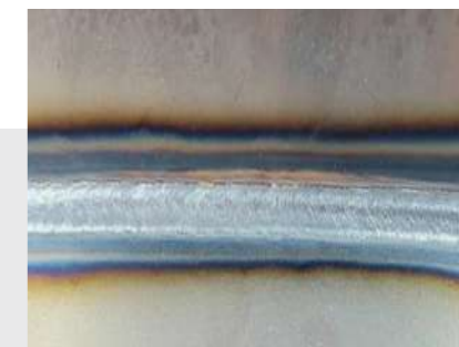
LSA (low spatter and low heat input)
